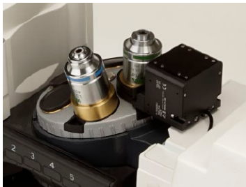
Matching spacer for same parfocal length / Slim cross-sections enable the use of directly adjacent lens mounts
