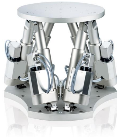
Fig. 3 Dynamic motion hexapods are used for motion simulation purposes, for example
