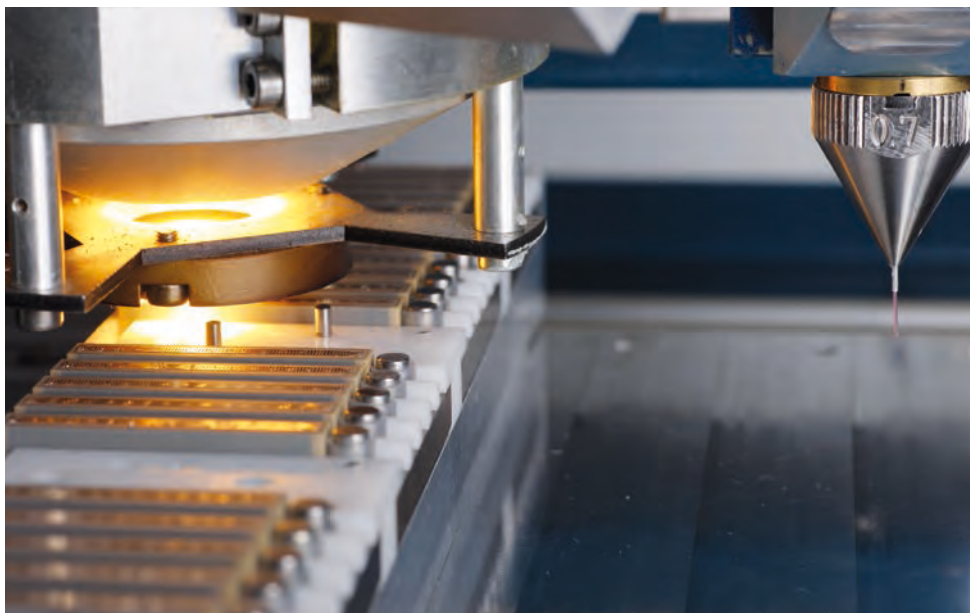
Automatic soldering machine with PICMA® actuators
