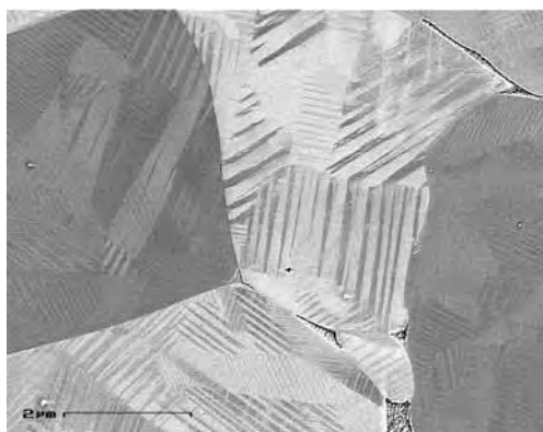
Fig. 2: A cross-sectional view of a ferroelectric ceramic clearly shows the differently polarized domains within the individual crystallites
